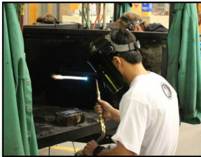
FIRE IT UP: Uriel Soto (9) is evening out the oxygen and acetylene outcomes for the perfect flame. "I like the hands-on work," said Soto. He planned to make two pieces of metal into one, and with a small lesson from Mr. Gutch, he succeeded. (Photo by Brandon Dearmore)
